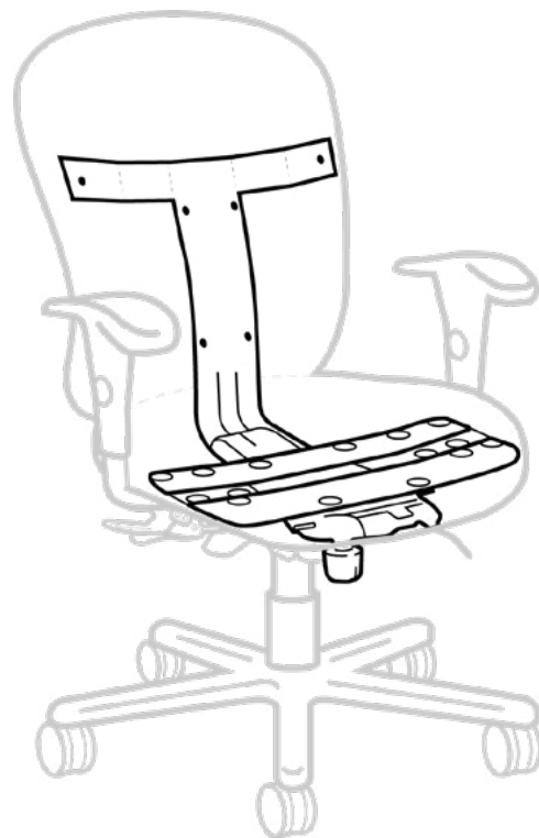
Steel Support Structure
